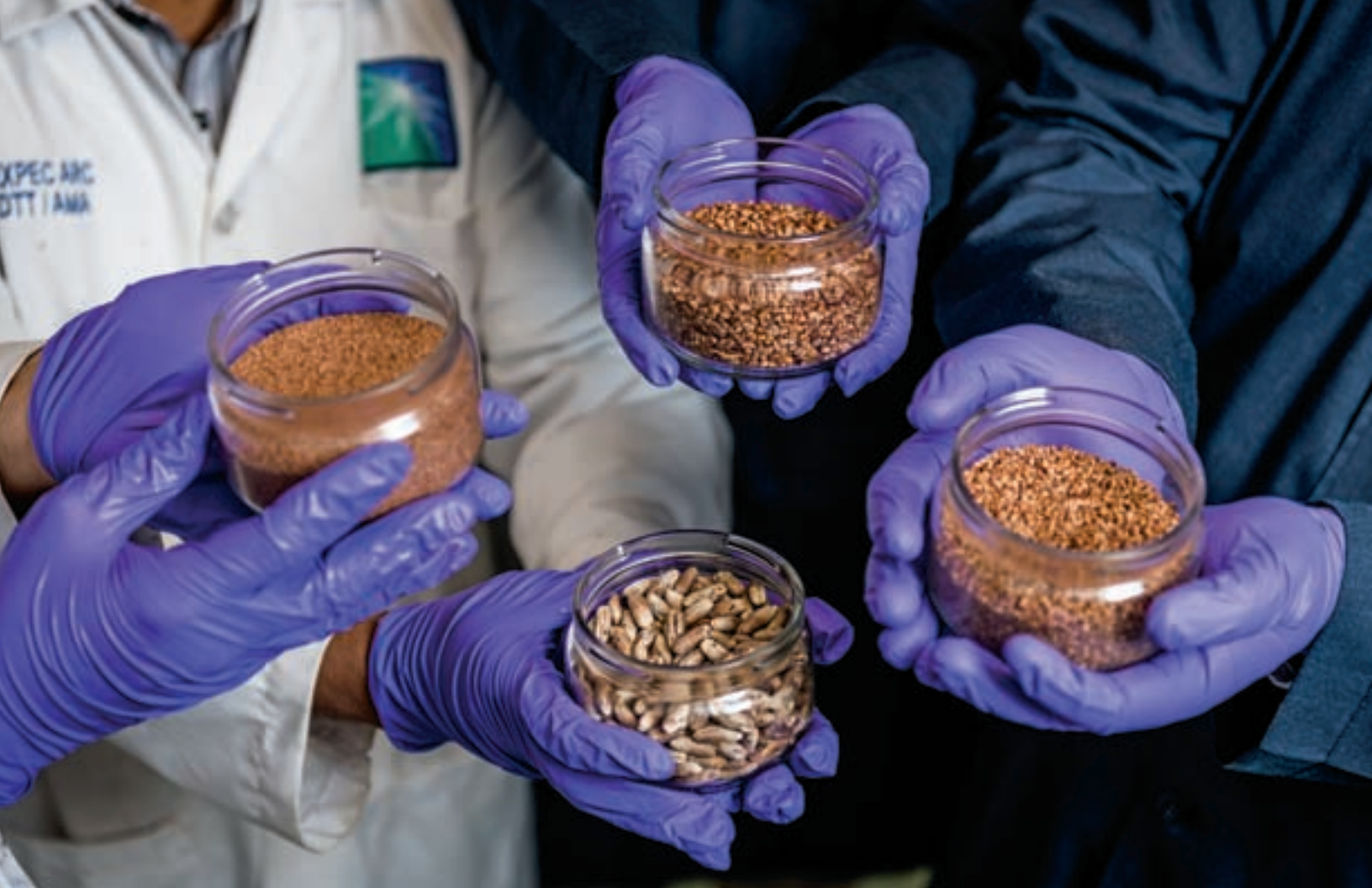
A display of whole date seeds, and several grades of ARC Plug products manufactured for laboratory evaluation.
