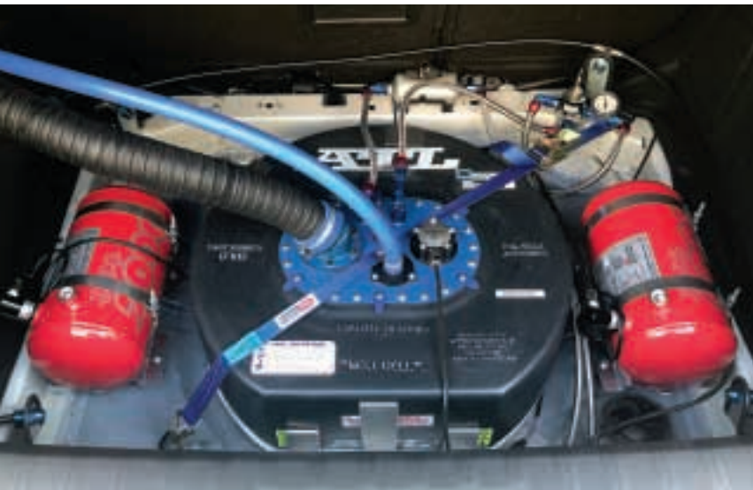
Left: A second fuel tank was added to the production Peugeot 308 passenger vehicle as part of the Octane-on-Demand system modifications. Bottom: The preliminary assessment of the Octane-on-Demand concept was undertaken using the single-cylinder engine testing facility in Dhahran.
