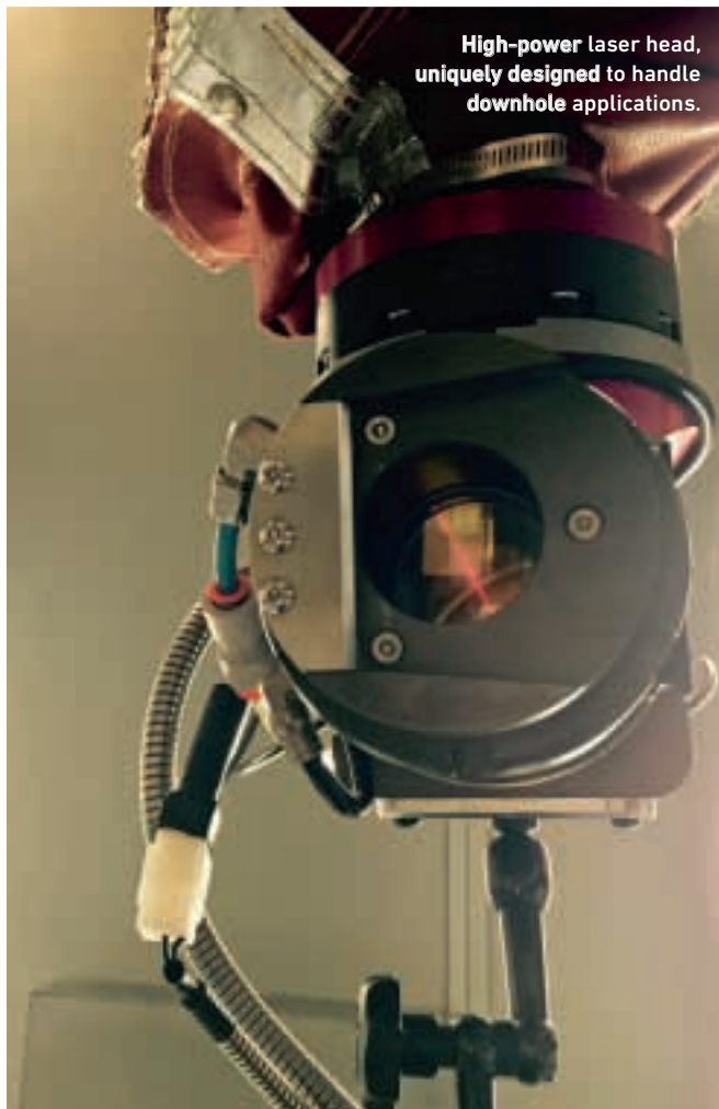
Lab experiment showing high-power laser perforation in rocks. The penetration is three seconds in length.
