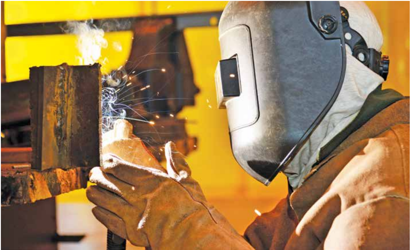
A worker remains protected while arc welding, which welds metals using the heat generated by an electric arc. (Photo Source: Saudi Aramco)
