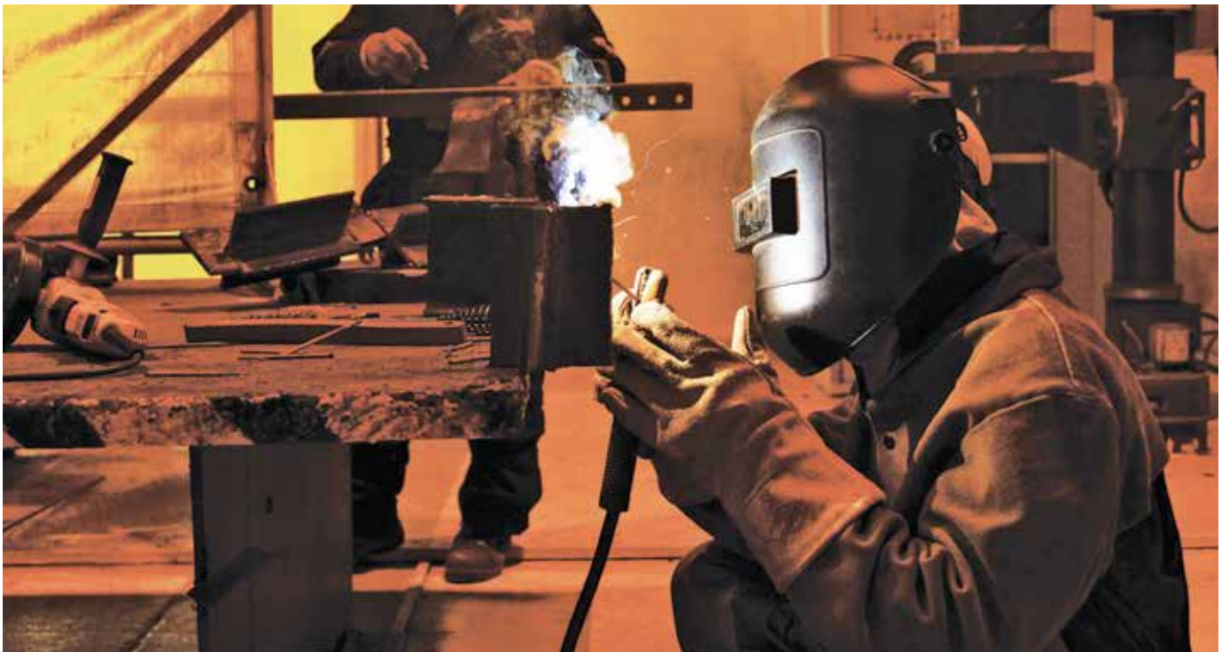
A worker demonstrates the proper way to engage in arc welding, which welds metals using the heat generated by an electric arc. (Photo Source: Saudi Aramco)
