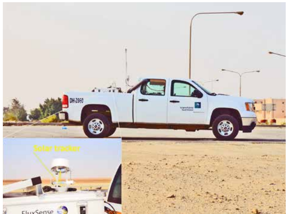
Figure 2. Solar Tracker. The solar tracker guides the sun light into the FTIR detector placed inside the white protective box. (Photo Source: FluxSense)
