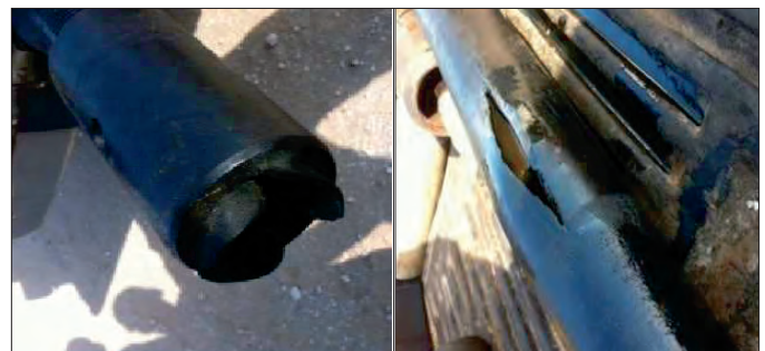
Fig. 2. Photos of the recovered broken prong.
