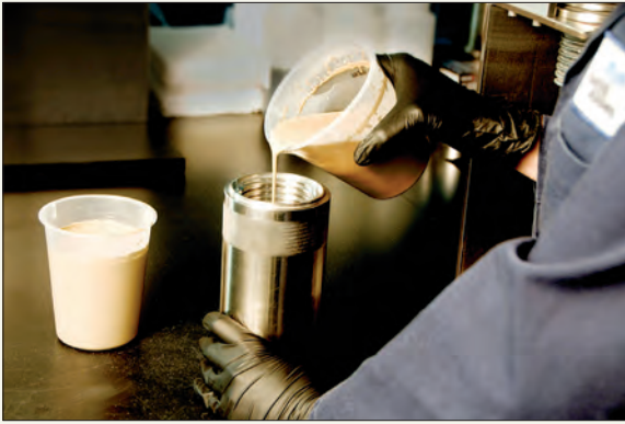
An engineer performing the mud check to confirm that the parameters meet the drilling program requirements for the well.
