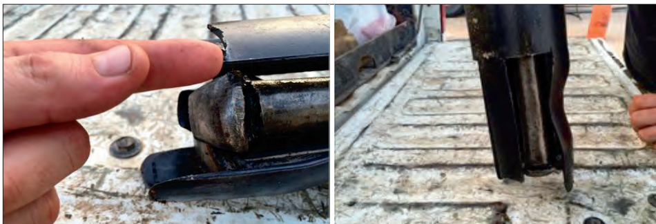
Fig. 3. Photos of the recovered modified pulling tool.
