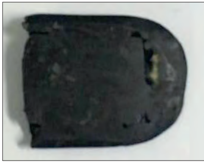
Fig. 4. A photo of the recovered latching dog.
