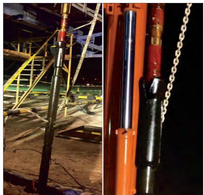
Fig. 8. Photos of the stuck plug from Well-A at the surface upon recovery.
