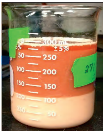
Fig. 13. The OBM with the sealing polymer after 30 minutes in a static state at room temperature.
