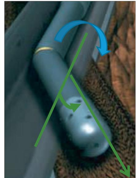
Fig. 4. MLT consisting of a controllable bent sub, movements depicted with arrows, and an orienting tool just visible behind it.
