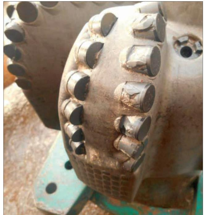
Fig. 19. Shear caps on a bit pulled out of the hole after reaching the casing point.
