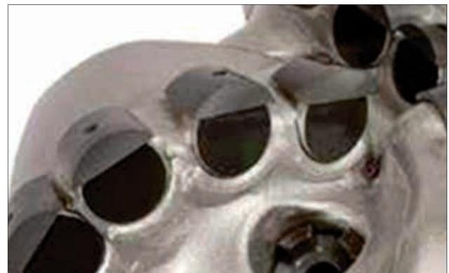
Fig. 9. Shear caps on a new PDC bit.
