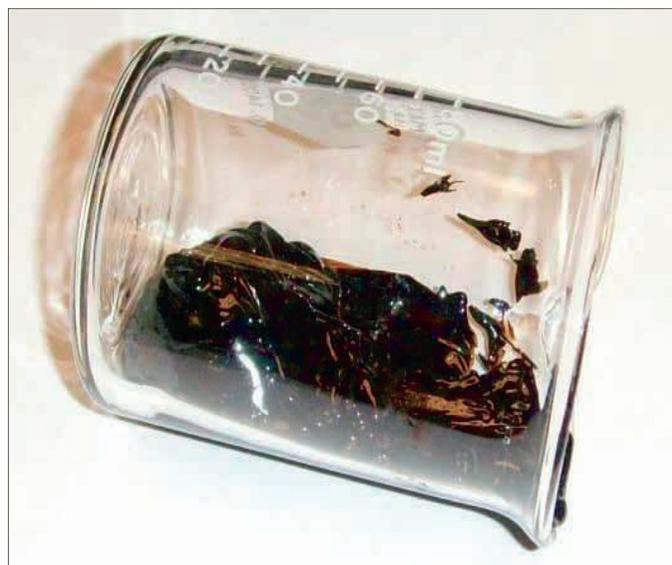
Fig. 7. Sludge sample after mixing.
