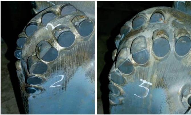
Fig. 20. Shear caps after completing a clean out job.
