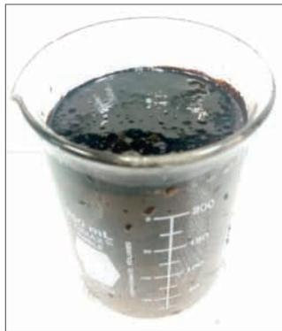
Fig. 18. Collected flow back sample showing viscous hydrocarbons.
