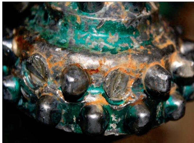
Fig. 3. Broken cutter teeth in an unpredictable pattern<sup>1</sup>.
