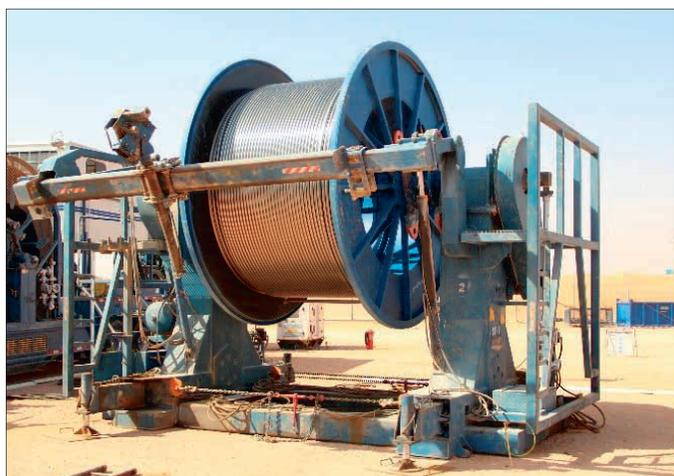
Fig. 4. Metal-jacketed ESP cable on location.
